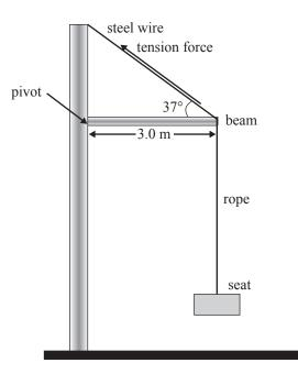
(i) The force exerted on the beam by the steel wire can be split into two components.
